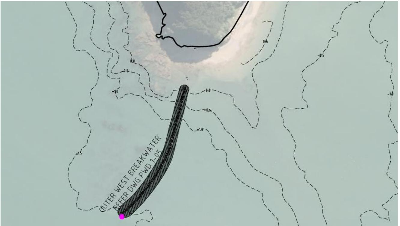
The proposed northern reef breakwater is to close the channel between Moutumarie Island and Taylors Island and is approximately 160m in length. The width at the base will be approximately 30m. The overall footprint of the structure occupies approximately 3800m<sup>2</sup> of the sea floor.
