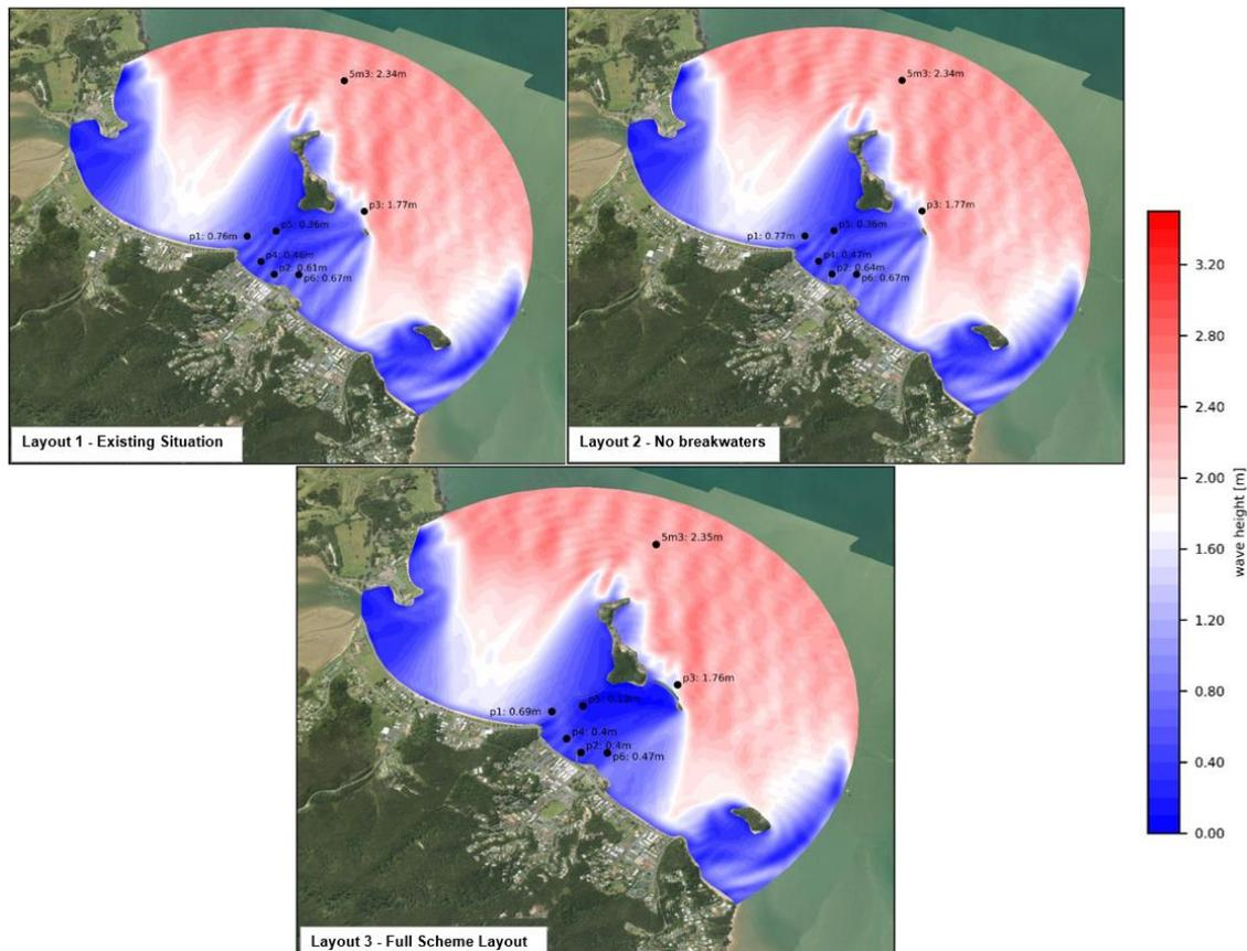
**Figure 1: Example of wave modelling results showing wave heights with existing and future layouts (adapted from MetOcean, 2021)**
